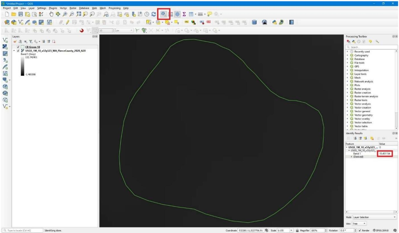
To improve the viewability of the LIDAR data in this small area, right click the layer name and go to properties, then the symbology tab. Change the min and max values of the black to white color gradient to 12 and 18. Now, elevations less than 12 appear all black and over 18 appear all white. You can navigate and zoom in around the LIDAR data. If you zoom in close enough you will see the edges gray of the pixels correspond to even values of meters in the projected UTM 10N coordinate system.
