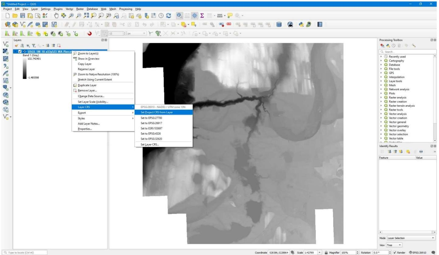
Check the coordinate system properties in the project file. Go to Project -> Properties to bring up the properties screen. Double, even triple check that the project CRS is the same as the LIDAR data CRS.
