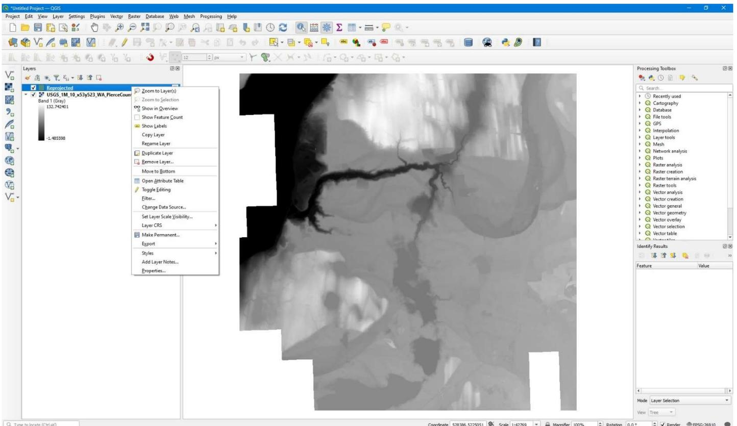
For vector layer files you will be using repeatedly and editing, I recommend saving them as a .shp file. Right click the layer name, go to Make Permanent. Save as an ESRI Shapefile file in the same directory. Then add the .shp file to the project and remove the temporary scratch layer. Zoom into the 18<sup>th</sup> green by right clicking on the project layer and then Zoom to Layer(s).
