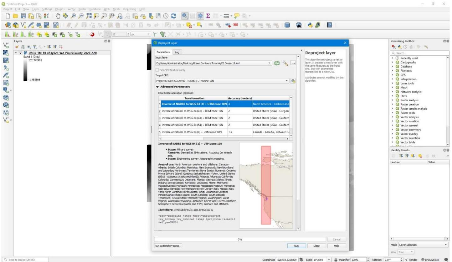
You will notice that QGIS added a temporary file to the Layers window called Reprojected. At the end of the layer name, you will see a computer processor type symbol; this means the layer is only temporary and will be discarded if not saved when exiting QGIS. Right click on the layer name to bring up the layer's options menu. Get used to doing this because a lot of the work we will be doing with layers can start from this menu.
