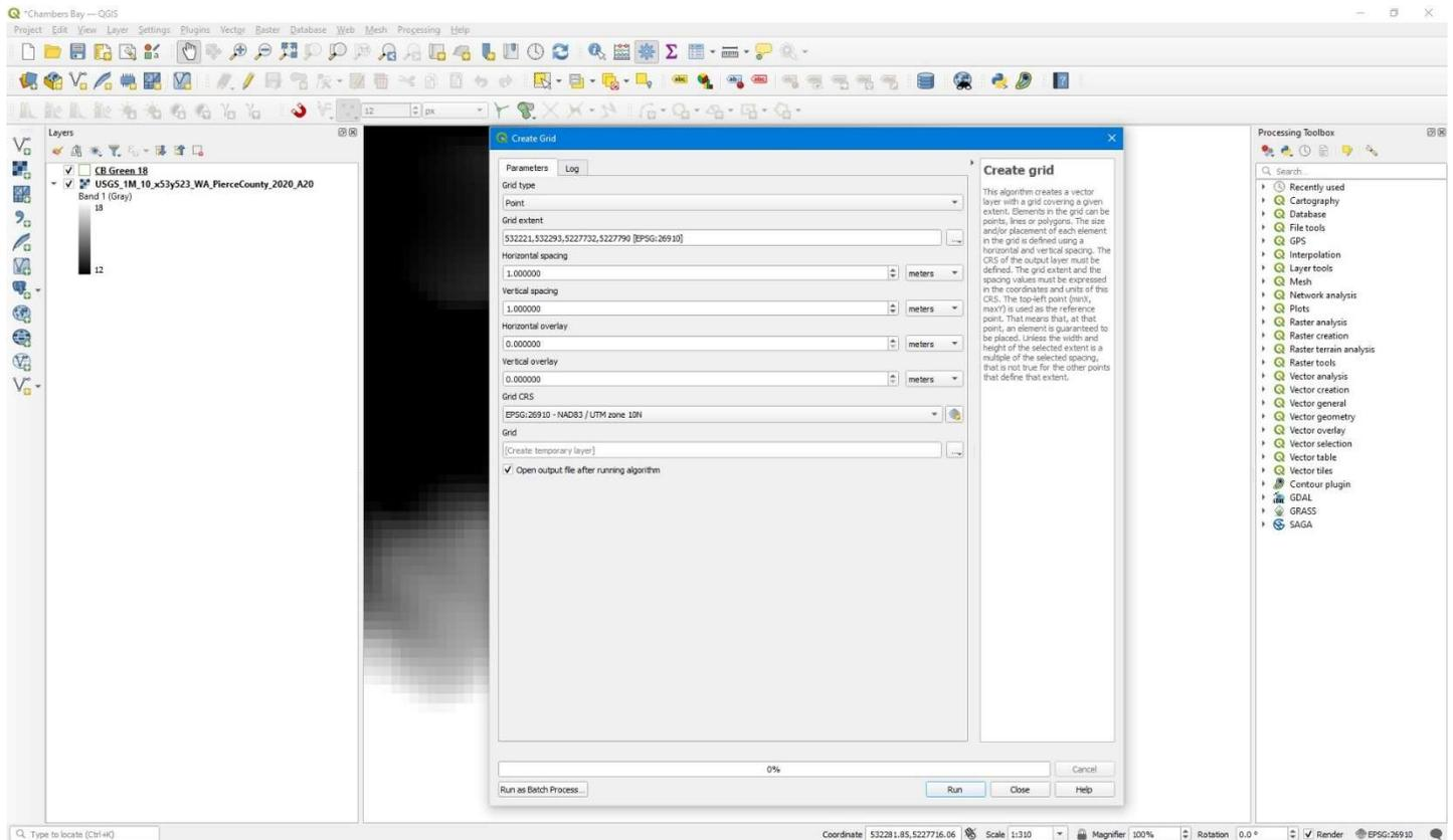
Now move the grid 0.5m in the X and Y direction to the center of the LIDAR pixels. To do this, type translate in the processing toolbox search box and under vector geometry click on the translate function that comes up. Select the grid we created as the input layer and type in 0.5 for the X and Y values for offset distance. Zoom in close to the pixels to notice that the new grid is now centered in the pixels.
