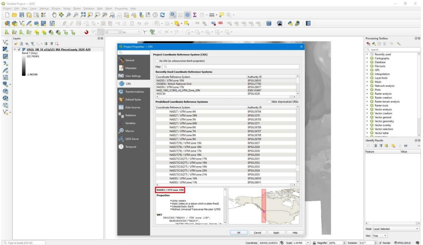
With the LIDAR data imported and project coordinate system set up, the next step is to add the Google Earth .kml file. Go to the menu item Vector -> Data Management Tools -> Reproject Layer. This brings up a window of options. Select the .kml file, set the coordinate system to Project CRS: ESPG:26910 – NAD83 / UTM Zone 10N.
